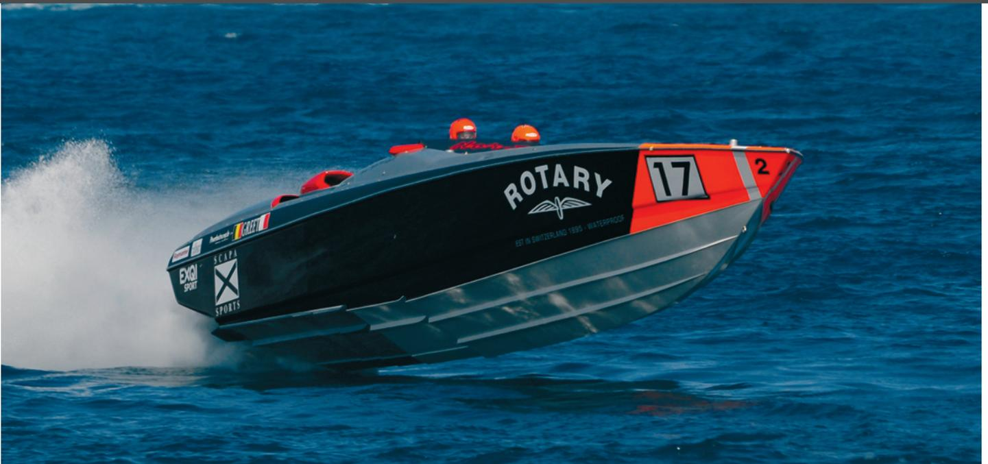
whisk compared to what I drive now. I now have two 600hp Mercury supercharged engines that drive a 41-foot boat."
